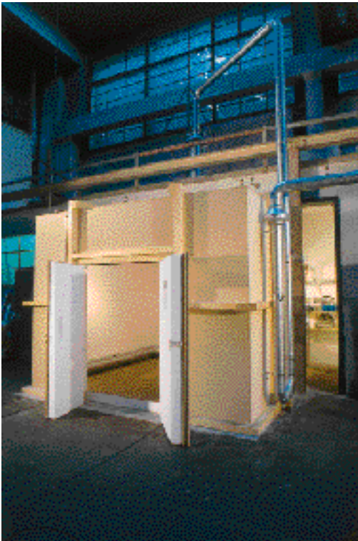
Figure 1 Test rig with calorimeter room and dilution tunnel to determine power output efficiency and emissions of solid fuel burning appliances at the Laboratories for Sustainable Energy Systems , Switzerland Photo Heiner Grieder, CH-4438 Langenbruck
