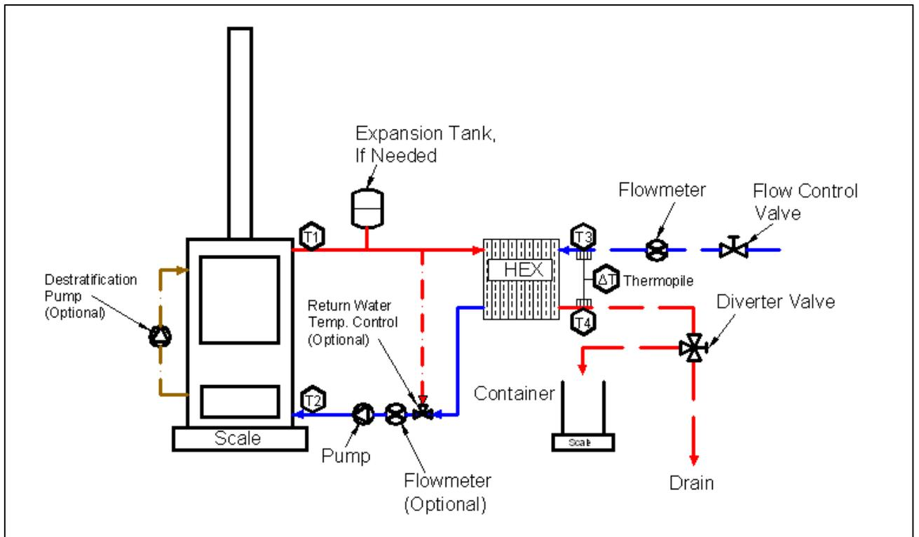
Note: Illustrated appliance pump location and flow path through the appliance are generic and may vary based on the unit being tested.
